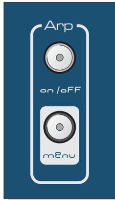
This section of eleVAta features the Arpeggiator. An arpeggiator is a device that takes the notes of a chord and, rather than playing them simultaneously, plays them one at a time in sequence automatically. Although some arpeggiators require programming in advance, most take their note data from a keyboard input, as this offers a more immediate interface.
