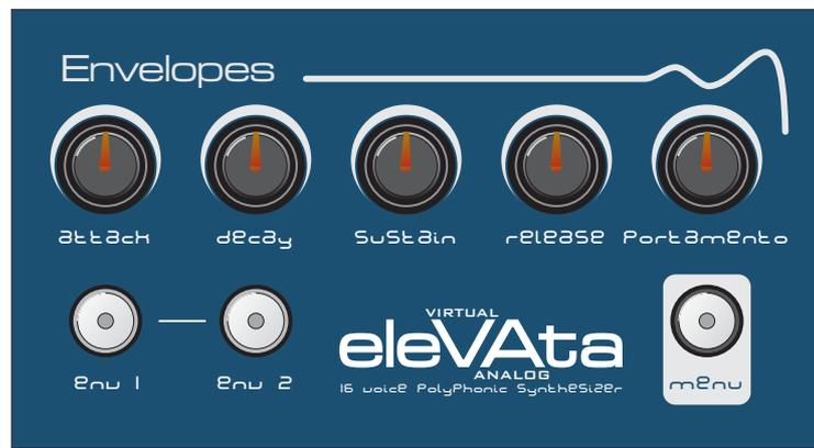
This section of eleVAta is used to shape the sound over a period of time with two envelopes available. The first envelope is fixed to amplitude (or volume) and decides how quickly the sound starts, sustains and then fades away. The second envelope can be used to control the filter frequency, pulse width or pitch modulations etc to alter the character of the sound.
