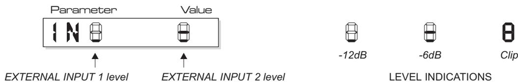
**6. Output Levels [OU]:** This function allows you monitor the audio output levels from the six individual [OUTPUTS] on the rear panel. The main display indicates the levels of all six outputs simultaneously in 6dB steps as shown in the following example:
