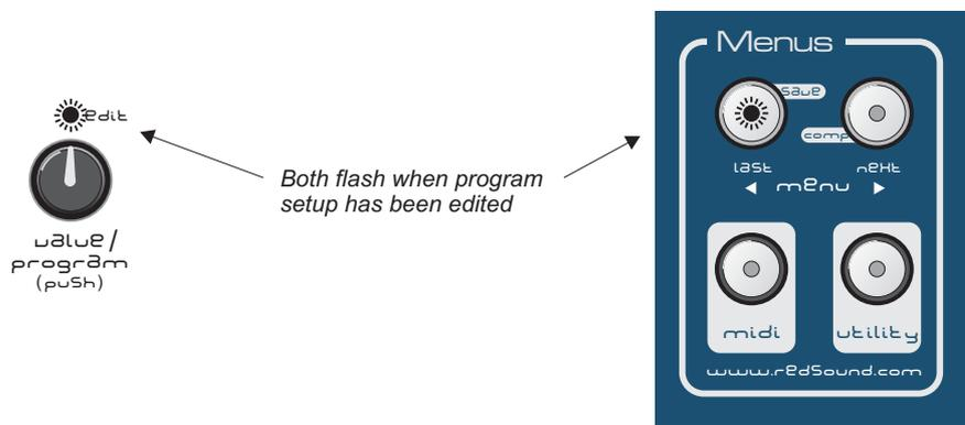
**NOTE:** The [SAVE] and [COMPARE] buttons are dual function (also control MENU selections) so, if any of the [MENU] functions are ON, the [SAVE] indicator will not flash and the [SAVE]/[COMPARE] functions will be inactive.
