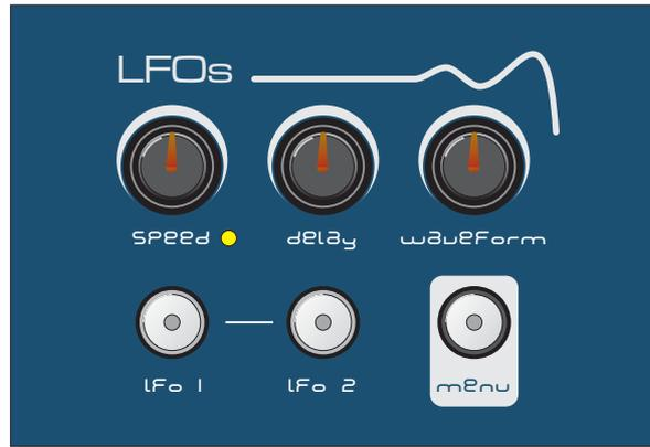
This section of eleVAta features 2 LFOs (Low Frequency Oscillators) which make regular electronic variations too low to be heard when converted into audio vibrations. They can be used independently to alter elements of the sound by adding vibrato or changes to the harmonic content.
