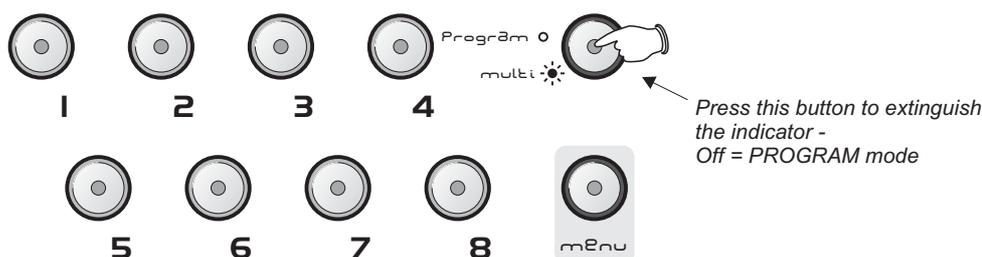
This button sets the basic operating mode for eleVAta. Each press will change the mode, the indicator within the button showing the status as follows:
