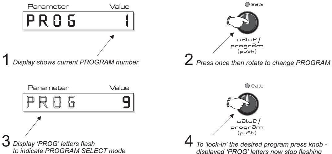
The 'PROG' section of the display will flash during program select mode. When you have found the sound you want, press the [VALUE/PROGRAM] encoder knob again to 'lock-in' the program.
