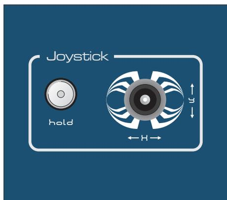
This section of eleVAta features a fully assignable joystick for multiple parameter manipulation. You can assign parameters such as filter frequency/resonance, oscillator pitch, ring modulation etc to the joystick for added creative expression and 'on-the-fly' editing. The joystick operates in parallel to the labelled front panel controls.
