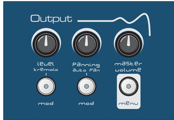
This section of eleVAta features various effects such as panning, chorus, flanger and tremolo. Each PART has its own level control whilst the master volume control governs the overall output level. The routing for the six individual outputs can also be set using the output MENU.
