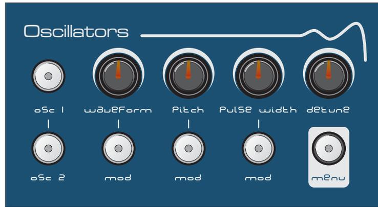
This section of eleVAta produces the musical tones which form the basis of subtractive synthesis. There are two oscillators per 'voice' (musical note), each producing audible vibrations to act as a sound source. The timbre of each oscillator depends on its harmonic content which is determined by the waveform. There are basically two waveforms available, SAWTOOTH and SQUARE each with its own specific set of harmonics.
