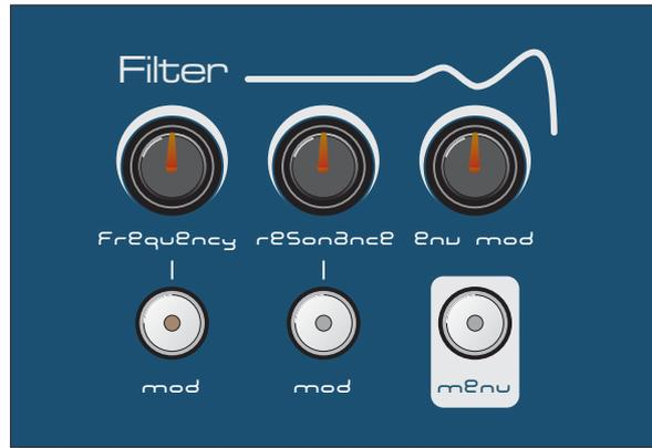
This section of eleVAta features a classic, smooth 12dB per octave filter which, in subtractive synthesis, is used to remove unwanted frequencies. There are three different types of filter to choose from, LOW PASS, BAND PASS and HIGH PASS or the filter can be totally switched off.
