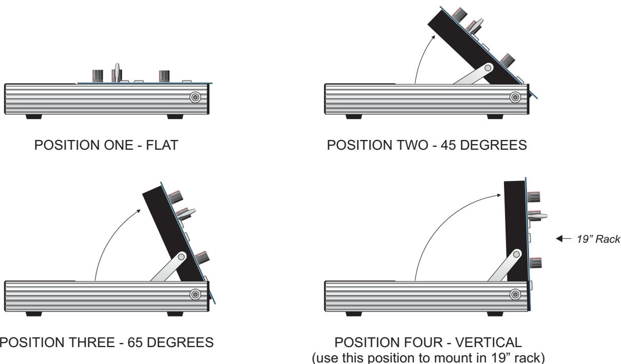
**LOWERING THE PANEL:** First you need to release the support arms from their locators. Tilt the control panel forwards then, using one hand at either side, lift the chrome supports with your index fingers simultaneously before lowering the panel backwards to the next set of locators, or all the way down to the flat 'parked' position. During panel movements like this you will need to keep continuous upwards pressure on the supports to avoid them dropping down into their locators.
