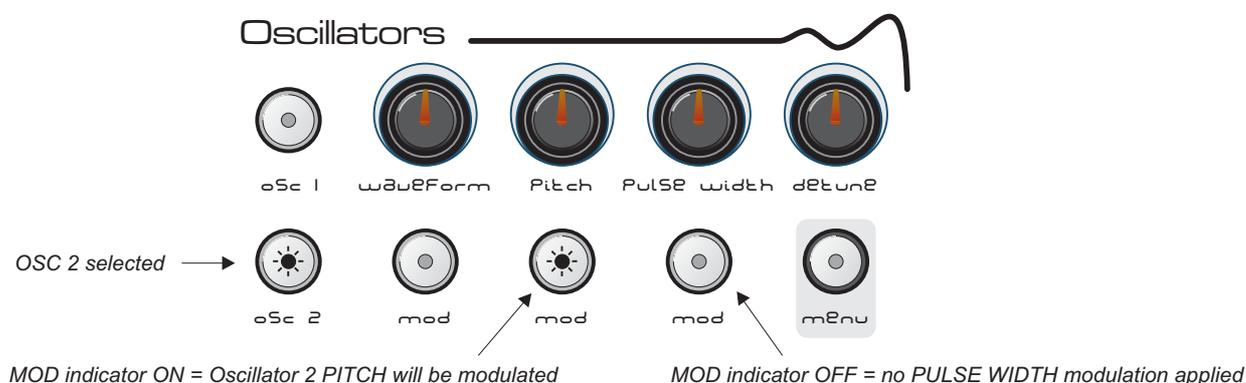
But what is modulating it, and by how much? In order to see and adjust modulation settings for a particular parameter, we need to activate Modulation Edit mode.
