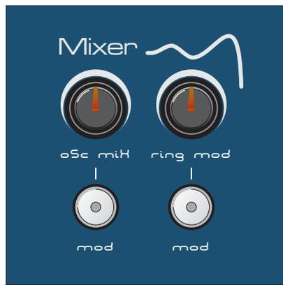
This section of eleVAta allows you to adjust the relative mix levels of the oscillators (or external audio inputs) and also add ring modulation. Ring modulation occurs when the two sound sources are multiplied together and this gives the sound a hard, overdriven edge.
