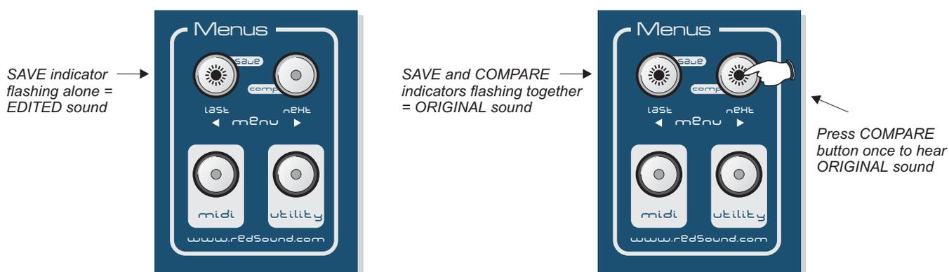
**SAVING TO A NEW PROGRAM LOCATION:** To save the edited sound in any other user program location first activate the [COMPARE] function, then use the [VALUE/PROGRAM] encoder to select a new program number and finally, press the [SAVE] button to store the sound, as shown in the following example:
